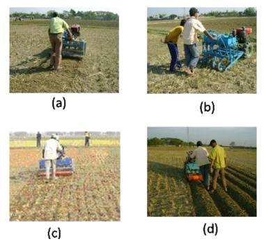
**Figure 2.** Two Wheeled Tractor Operated seeder (PTOS) in Bangladesh; planting six rows in no-tilled field in full-width tillage mode (a), No-till tined drill planting rabi crop (b), strip-till planting crop (c), forming raised bed and planting simultaneously in no-tilled field (d).
