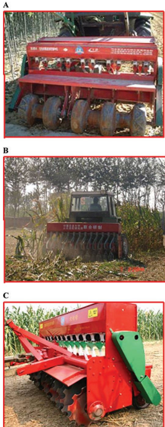
Figure 6. Three typical active antiblocking no-tillage seeders. (A) 2BMFS-5/10 no-tillage seeder; (B) 2BMDF-12 no-tillage wheat seeder; (C) 2BDPM-12 no-tillage wheat seeder.
